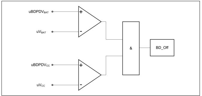
Figure 24 Logic diagram of BD\_Off detection
