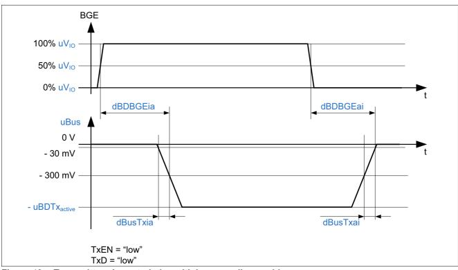
Figure 43 Transmitter characteristics with bus guardian enable
