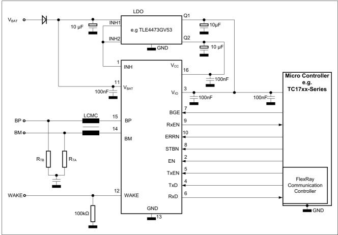
Figure 50 Simplified application example for the TLE9221SX
