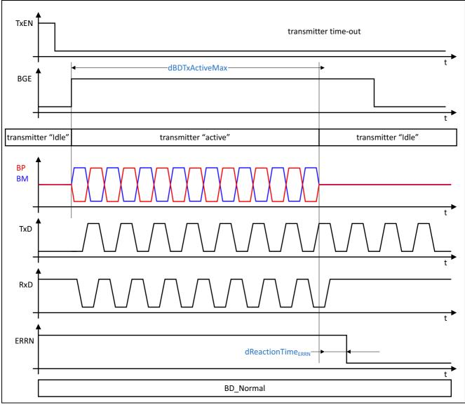
Figure 39 Transmitter time-out function
