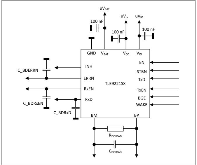
Figure 40 Simplified test circuit
