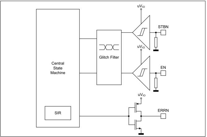
Figure 9 Block diagram of the Host Interface
