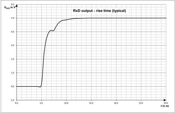
Figure 47 RxD output rise time (typical simulation value)
