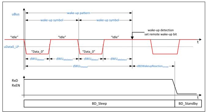
Figure 18 Standard wake-up pattern
