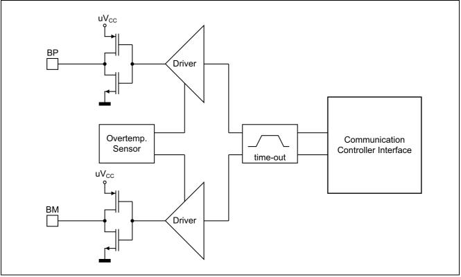
Figure 4 Block diagram of the Transmitter
