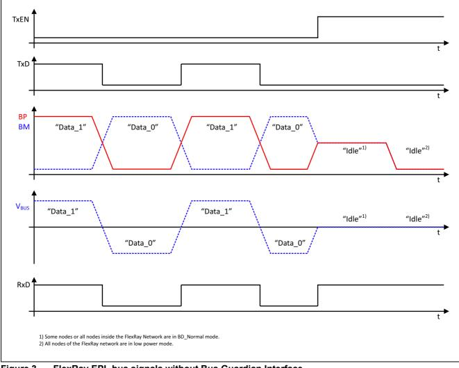
Figure 3 FlexRay EPL bus signals without Bus Guardian Interface
