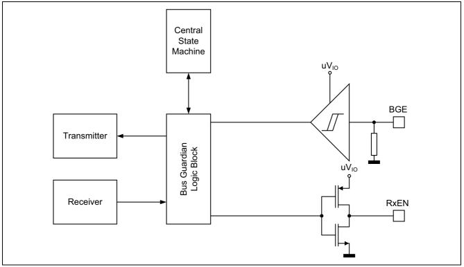
Figure 8 Block diagram of the Bus Guardian Interface
