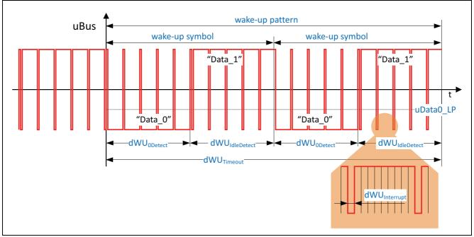
Figure 20 Wake-up by payload
