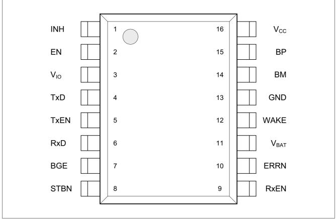
Figure 1 Pin configuration
