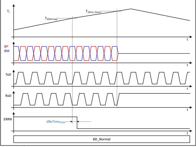
Figure 38 Overtemperature protection
