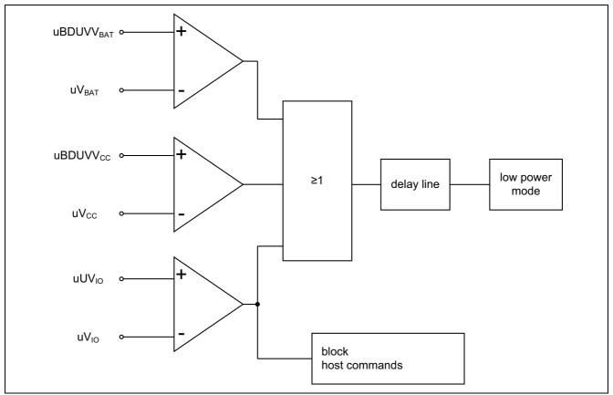
Figure 23 Logic diagram of undervoltage detection
