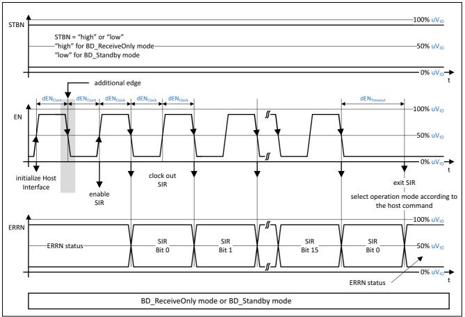
Figure 12 SIR readout in BD\_ReceiveOnly or BD\_Standby mode
