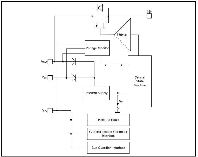
Figure 21 Block diagram of Power Supply Interface
