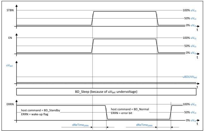
Figure 13 Status at the ERRN while uV<sub>BAT</sub> undervoltage
