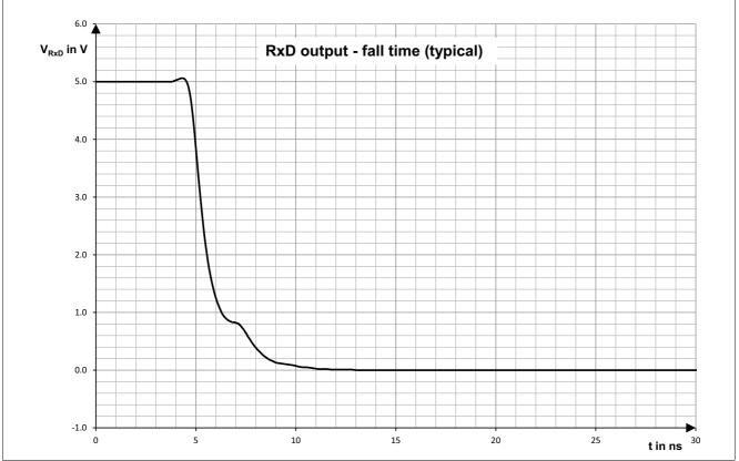
Figure 48 RxD output fall time (typical simulation value)
